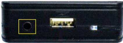
External AUX input via 3.5mm jack connection for connecting external audio sources such as:
