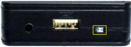
Wireless connection via Bluetooth for audio streaming via A2DP complete with charge function possibility (via USB port).
