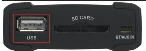
Input for connection of an USB source. Controls of the USB source via the original buttons of the radio or steering wheel controls.
