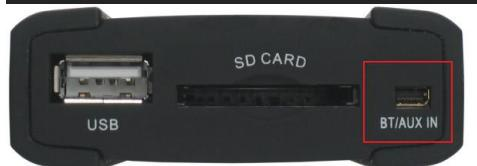
Input for car kit Bluetooth module (optional). This bluetooth interface makes it possible to the iPod interface or USB/SD interface to expand with Bluetooth audio streaming and/or Bluetooth car kit function. This makes it possible to get a phone with A2DP (Advanced Audio Distribution Profile) and HSP (Headset Profile) to pair with the radio system for audio streaming and car kit via Bluetooth feature on library level.
