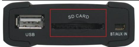
Input for connection of an SD card. Controls of the SD card via the original buttons of the radio or steering wheel controls.
