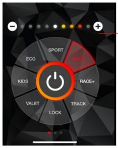
**Profile fine adjustment**Each driving profile can also be reduced or reinforced by 4 steps.
