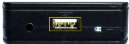
The NavInc Bluetooth interface has a USB port for charging connected devices.
