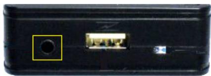
External AUX input via 3.5mm jack connection for connecting external audio sources such as:
