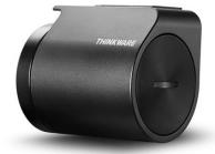
The dash cam is on standy until a movement is detected. When the Radar Module detects a movement, the dash cam wakes up and gets ready to record. If an impact is detected, a 20 second video (10 seconds before and 10 seconds after the impact) is saved.
